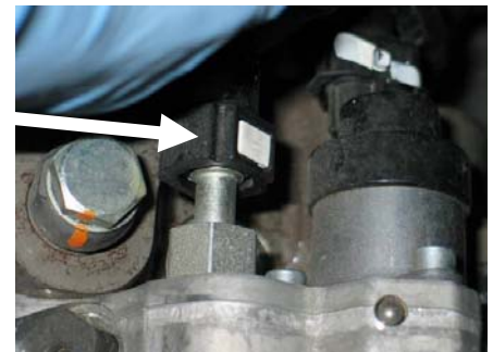
Step 6 - This is a photo of the OEM quick connect fitting that will be disconnected apart from the pump. Once disconnected, adapt the Fitch 2” male hose to the OEM female feed line & the Fitch 24” female quick connect to the OEM male off the injector pump.
