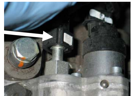
Step 6 - This is a photo of the OEM quick connect fitting that will be disconnected apart from the pump. Once disconnected, adapt the Fitch 2” male hose to the OEM female feed line & the Fitch 24” female quick connect to the OEM male off the injector pump.
