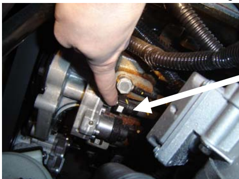
Step 6 - This is a photo of the OEM quick connect fitting that will be disconnected apart from the pump. Once disconnected, adapt the Fitch 2” male hose to the OEM female feed line & the Fitch 24” female quick connect to the OEM male off the injector pump.
