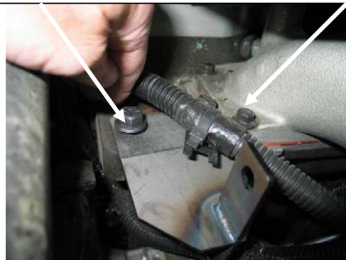
Photo #2 - Here is the photo of the metal bracket mounted – use existing bolt on truck & additional one is included in kit to self tap in the empty
