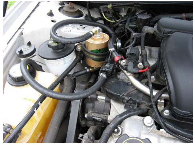
Using Fitch white plastic disconnect tool, separate the OEM male from OEM Female on the fuel rail
