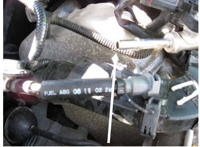
Using Fitch white plastic disconnect tool, separate the OEM male from OEM Female on the fuel rail
