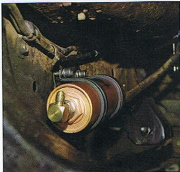
The Fitch was mounted along the frame with straps provided in the kit, and the fuel lines were connected.
