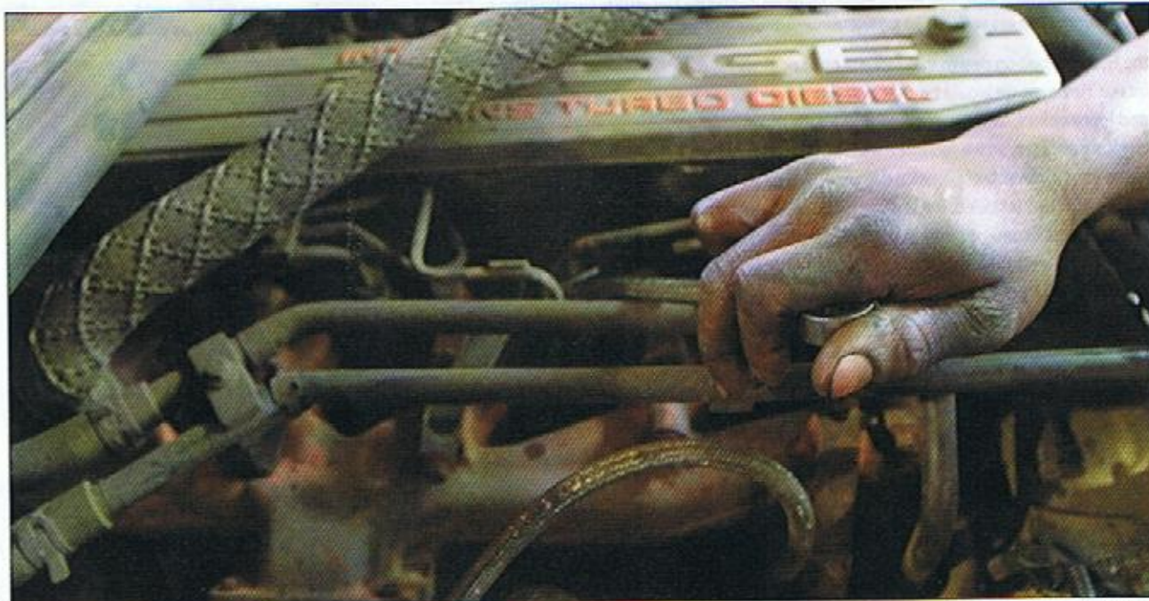
The Fitch was mounted along the frame with straps provided in the kit, and the fuel lines were connected.
